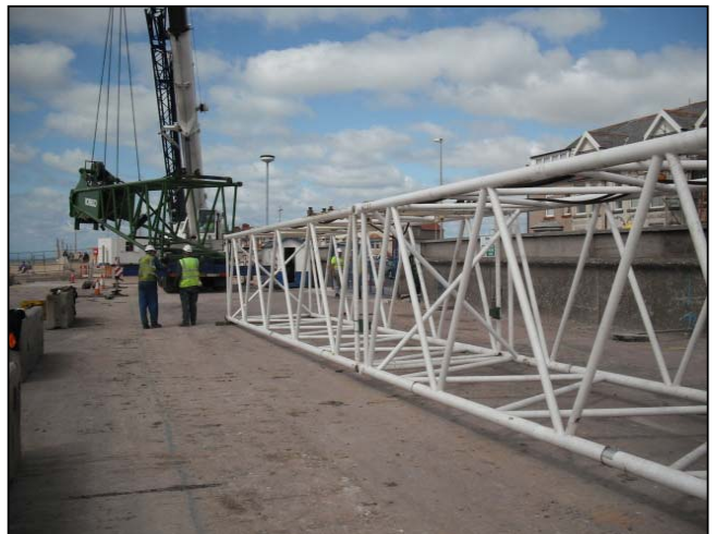
The last section of the crane jib being lifted into position for assembly.
